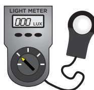
Fig 3.4 Light meters are used to check if all foliage is receiving enough light and if lamps have degraded.
